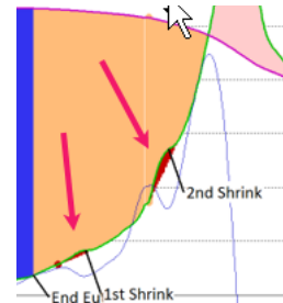
Figure 8 0.25% Shrink (two arrests)
