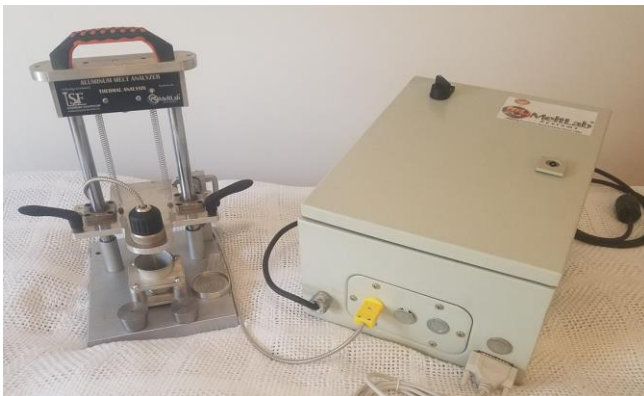
Stand with sample cup, Converter box, sample A356 curve with all results
